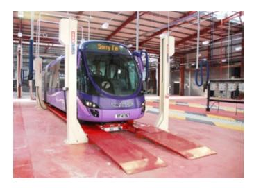
The wide platforms have an extremely low drive-on, ideal for low clearance vehicles, such as public transport buses. The standard approach ramps have a stream-lined effective design.
