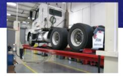
The Stertil-Koni ST 4175 and ST 4250 vehicle lifts are very versatile and powerful Ultra 4-Post platform lifts. They are widely suitable for any workshop situation. The design ensures maximum working ergonomics under and around the vehicle. Mechanics can work comfortably standing upright and have optimal access to the vehicle and any necessary vehicle maintenance equipment, such as, Axle Stands, Transmission Jacks and Jacking Beams.
