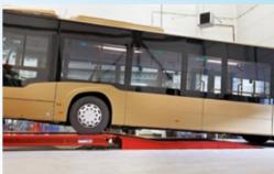
SKYLIFTs as either two individual lifts or a single lift. In doing so, vehicle configurations of up to 100 feet in length and with a total weight of up to 156,000 lbs. can easily be lifted! The SKYLIFT is even flexible with regard to its width. During installation, the width between the platforms can be adjusted to your particular vehicles.
